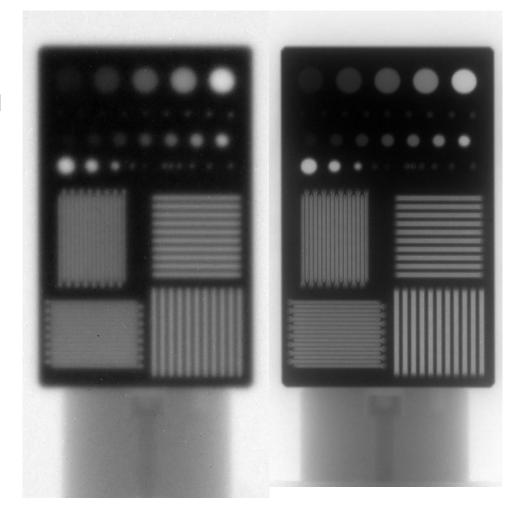
New PE/ZnS:Ag based scintillation screen.
