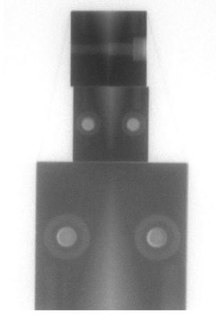
Tomography of different metal parts have been tested and work fine. Due to round edges the resolution seems to be lowered.
